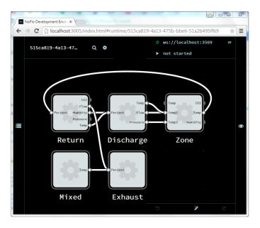
Fig. 3. Flow-based configuration environment that let communication between field devices be visually parameterized (on this example, connections have no precise meaning). The components represented here were automatically generated from the sections of the Air Heating Unit of our test case. Inputs and outputs are data points.
